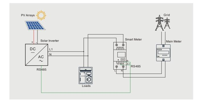
Smart meter measures and calculates the system electrical parameters and interacts with inverter for energy management and zero export control purpose.
