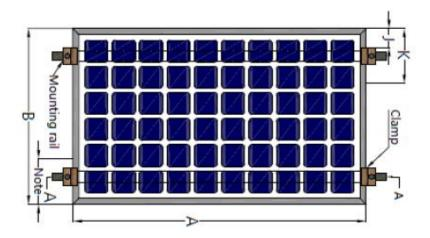
Using this mounting method will refer to following mechanical load value based on IEC 61215 standard considering to 1.5 times safety factor:
