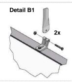
Tighten the hinge bolts B1 <u>by hand</u>. These must be removed temporarily in Step 4.
