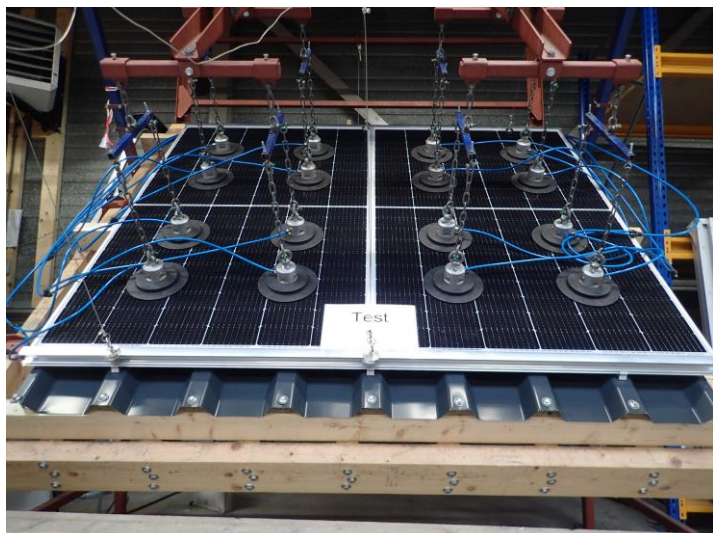
Photo 9 The suction cups are placed in position and test specimen 1 is ready for testing.
